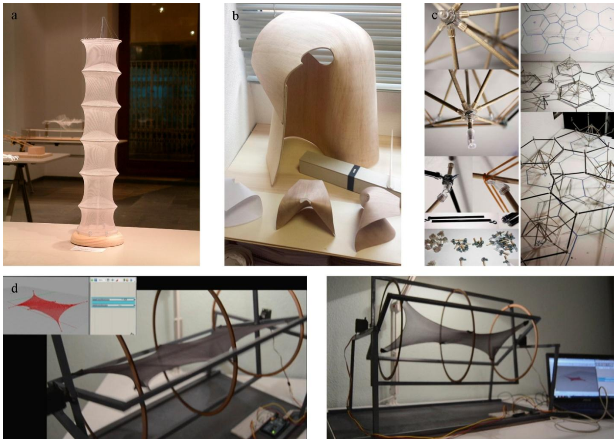
Figure 2. (a) Proposal for tensile structure; (b) Stool scale 1: 1 with curved wood; (c) Three-dimensional model of variable structure; (d) Structural model of tensioned fabric in movement using Processing.
