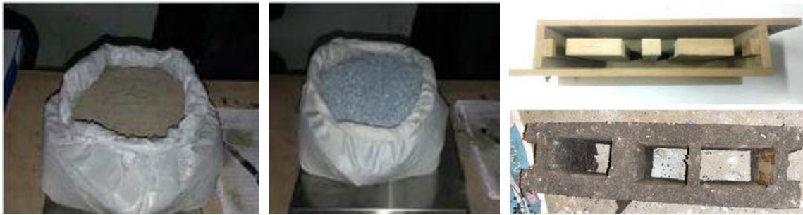
Fig. 4. (a) River bed sand; (b) Plastic pieces; (c) Manufactured hollow brick and mold [17].
