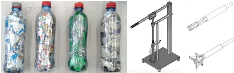
Fig. 2. (a) Eco-brick samples (from left to right: with tetra pak metal, PET, paper, and cardboard fillers) [16]; (b) The mechanical waste compactor [30].
