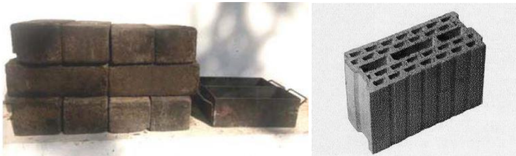
Fig. 3. (a) Plastic-sand brick [17]; (b) Ecobrick® ceramic brick [34].
