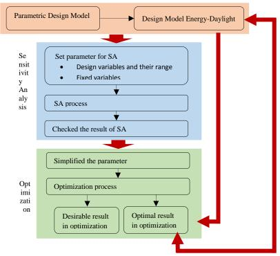
Figure 2: The procedure of the proposed method for the simulation process.
