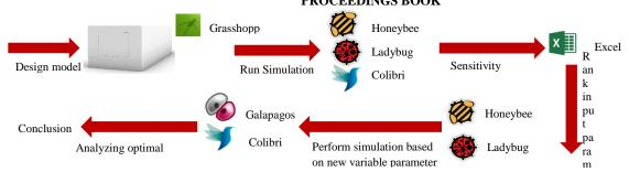
Figure1: Sensitivity-based building design optimization
