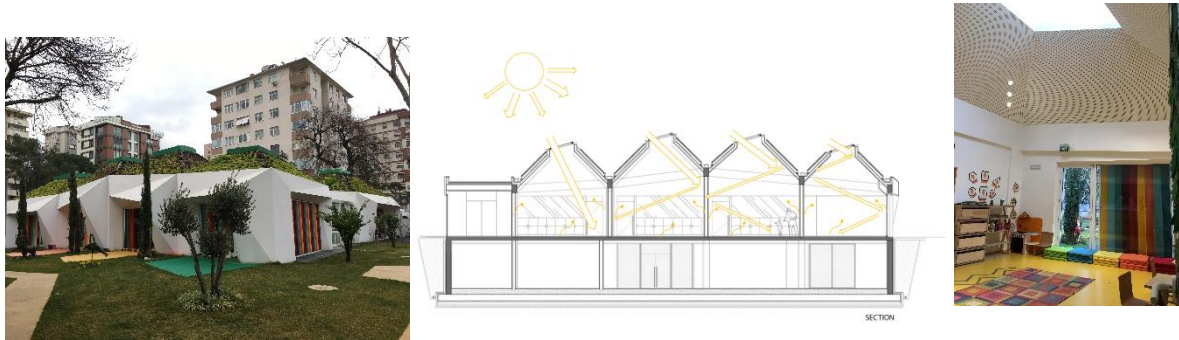
Fig. 2.3 (a) Bahriye Üçok Nursery School South-Western Façade, Dilekci Architecture, 2016, Istanbul, Turkey; (b) Passive Solar System Utilization by Means of Roof Lights of Bahriye Üçok Nursery School (c) Bahriye Üçok Nursery School Learning Area
