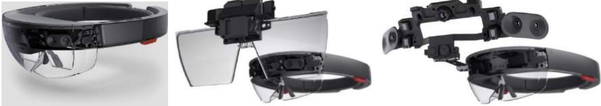
Fig. 2. (a) holographic platform computer; (b) optic see through lenses; (c) sensors [5]
