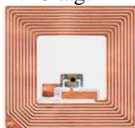
Figure 5. A passive NFC tag [2]
