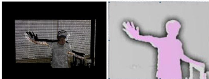
Fig. 4. kinect 3D image reconstruction: (a) 3D image; (b) depth map
