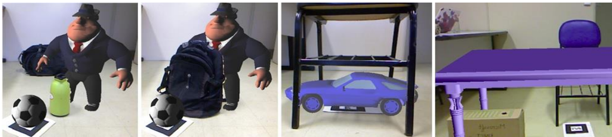
Fig. 9. (a) Real objects behind and between the two virtual objects, (b)Virtual object between real objects. (c)Virtual table rendered over a real chair and a real object between the virtual object.
