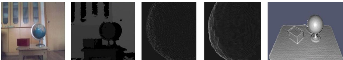
Fig. 8. 3D depthmap processing – (a) Raw depth map and color image, (b) Point-clouds generated from fused Model and from raw depth map, (c) The complete model.
