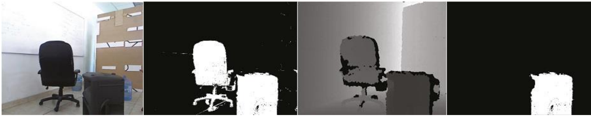
Fig. 10. (a) RGB color image (b) Initial mask. (c) Depth image (d) Resulting image segmentation.
